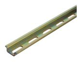
DIN15 rail with 15x5.5x1 mm, made of galvanized steel, with a 6 mm² copper cross section, with fixing slots, 2 m length
