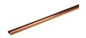
DIN rail DIN32, universal carrier made of a sheet metal profile in electrical engineering for fastening electrical equipment in distribution boxes, control cabinets, junction boxes, etc. Different components (for example relays, impulse switches, timers, circuit breakers, terminal blocks) can be slid onto a carrier rail from the side or plugged on and locked from the front. The assembly of control cabinets and switch boxes is facilitated by this standardized method, which reduces labor costs.
