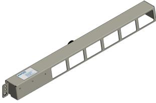
made of galvanized sheet steel 1.5mm with knurled screw for lateral fixing in the trunking shell. Dimension: 525x47(53)x40mm Color: RAL 7032 pebble gray Equipped: 1 pcs. blind hole clamp 10x2.5mm <sup>2</sup> 10128
