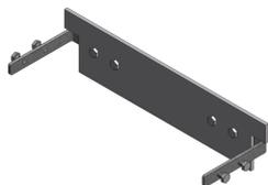
made of sendzimir-galvanized steel sheet 1.5mm with protective edge height 0 in special aluminum profile Woertz pressed in groove and impact sound trapezoidal rubber as cover support including connecting material height 50mm / nominal cover width 200mm
