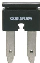
Insulated cross connector, for tension spring terminals 12mm for staggered connection of adjacent terminals. 20.6x5.2x35.1 mm
