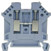
Terminal block DIN35 2.5mm<sup>2</sup> 46x6x43mm gray with best possible contacting, stainless steel screws, 4-digit marking possibility on both sides, recessed for cross-connections
