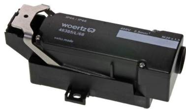
Junction box 5P(4mm²) IP66/68 for Flat cabel IP 5G6mm² With fastening
